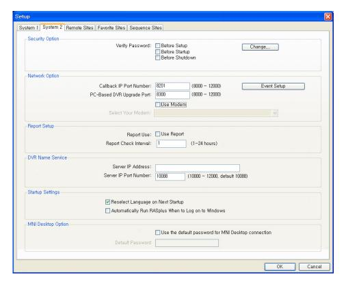
**System 2:** Set up the modem connection information for remote access, system password, network option, report function and DVRNS server.
