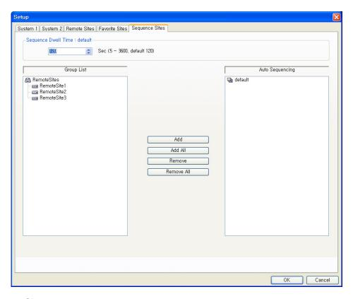
**Sequence Site:** Configure the sequence site. RASplus connects to the registered sites sequentially allowing connection to more than one remote site. Register an Auto Sequencing group and add desired sites in the Group List to the Auto Sequencing group. Video from the sites added to the Auto Sequencing group is displayed on the screen in the preset sequence interval during the sequence monitoring.
