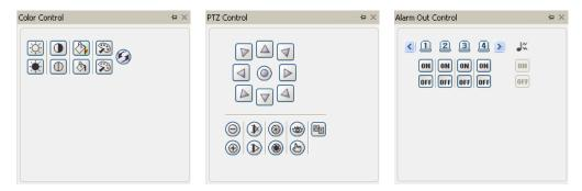
Three panels allow color control, PTZ control and alarm out control while live monitoring a remote site.
