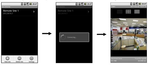
2. Push the Menu button of the device and a camera menu is displayed at the bottom of the screen. Tap the camera menu and select a desired camera from the camera list. Video from the camera is displayed on the screen. Dragging the screen to left or right moves to the previous or next camera group as long as there is video for these groups in the current screen layout.
