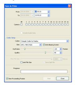
NOTE: Selecting *Include Audio Data* includes audio data when saving video with recorded audio. This option is not available when more than one camera is selected.
