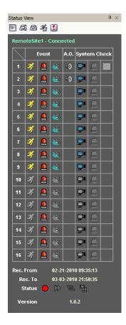
RASplus provides a status display, remote setup, system log and event log view of the connected remote site in real-time. To display the status of the remote site, select a camera or a site from the Remote Site list and drag it to the Status View panel. You can also select Connect Status from the popup menu displayed by clicking the right mouse button after selecting the site from the Remote Site list.
