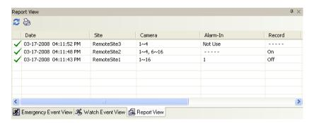
The Report View panel displays the system status information of remote sites. RASplus checks the remote site and reports system status. Clicking the cion on the panel reloads the data and clicking the cion prints the report out. Report Setup must be configured during RASplus System setup for this feature to function. Refer to 3.3 Menu – System Menu for more details.
