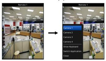
3. Push the Cancel button of the device to monitor video from other DVRs. The current connection is released and the default menu is displayed.
