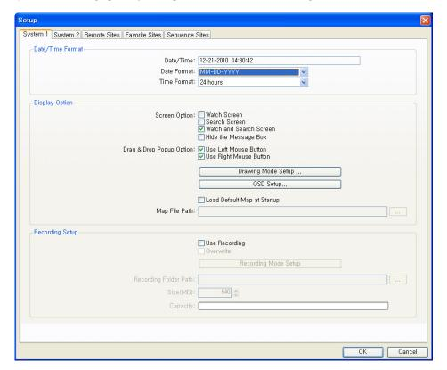
**System 1:** Set up the date/time format for RASplus, display option, and panic recording function.
