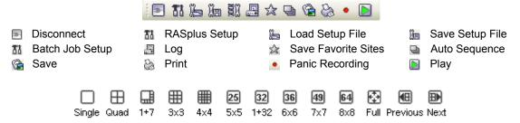
Select the desired screen layout using the layout toolbar. When changing the screen layout, the selected camera on the current screen will be located in the first cell of the new layout. When in one of the multi-view formats, clicking the 📵 or 🗈 button will move to the previous or next page.
