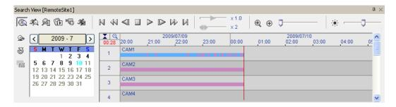
The Search View panel allows time-lapse or event searching of recoded data on the remote DVR.
