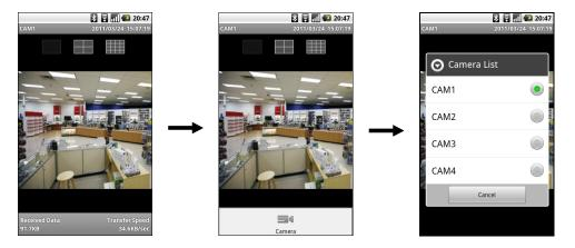
3. Push the Cancel button of the device to monitor video from other DVRs. The current connection is released and the default menu is displayed.
